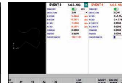
Auto Geometry Engine® software to calculate missing data for you as you program
