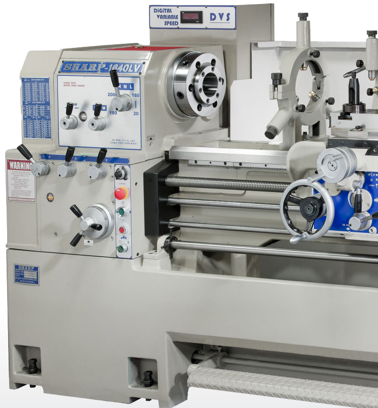
1640LV Digital Variable Speed Drive
